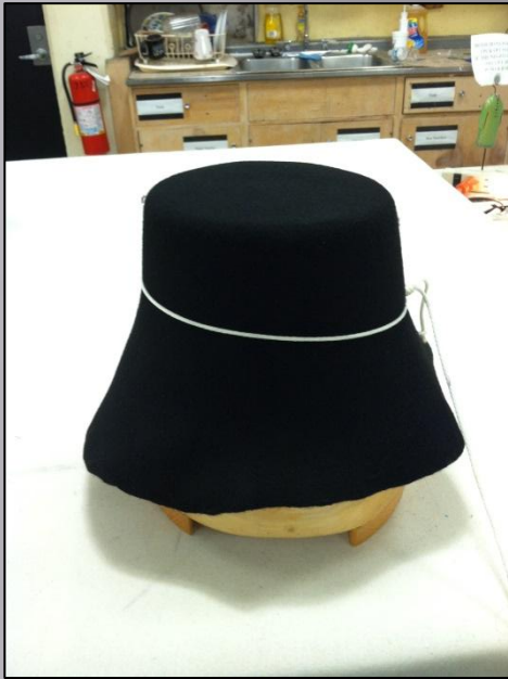
Shape felt hood over head block
