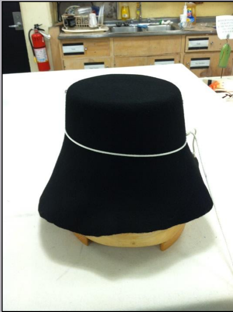
Shape felt hood over head block
